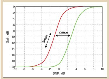
**Figure 1.** An example of the gain curves of Woods's single-microphone noise-reduction algorithm. The SMNR parameters represented by the green line have the same slope value as those shown by the red line, but a higher offset value.
