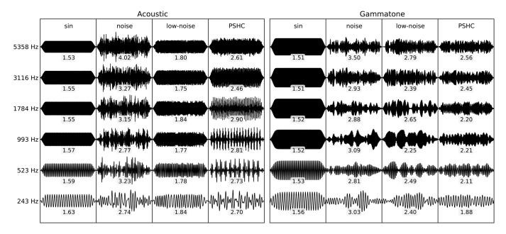
FIG. 2. Left panel: Acoustic waveform of the carrier signals used in Experiment 2 for each of the six frequency bands specified by their center frequency. Each segment shows 100 ms of signal. The number below each waveform is the crest factor. Right panel: Same but showing the output of auditory filters (linear fourth-order gammatone filter) centered on the center frequency of the band.
