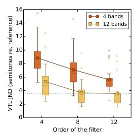
FIG. 4. (Color online) VTL JNDs for 4- (circle) and 12-band (square) vocoders as a function of filter order from shallow (4th order) to sharp (12th order). See Fig. 1, lower panel, for a description of the elements of the boxplot.
