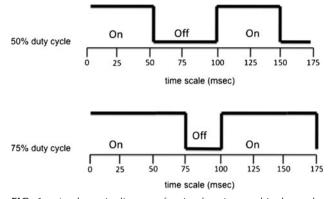
**FIG. 1.** A schematic diagram of gating function used in the study, shown for 10 Hz interruption. The *top panel* shows the square-wave gating function with the 50 % duty cycle, i.e. with 50 % on-duration and 50 % off-duration. The *lower panel* shows the same with the 75 % duty cycle, i.e. with 75 % on-duration and 25 % off-duration.
